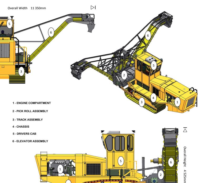
Engine: Caterpillar C6.6: 129 kW @ 2200RPM
